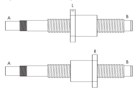
Example 1. Nut flange left position with standard machining – ALB
