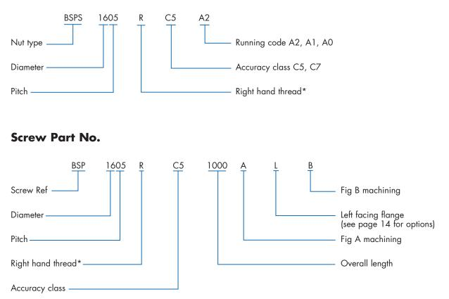
\* Some screws are available with left hand threads, these are clearly marked in the data/dimension tables. To specify a left hand thread use designation L instead of R
