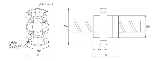
SD - Screw dia, P - Pitch, K - Stiffness (N/µm)
