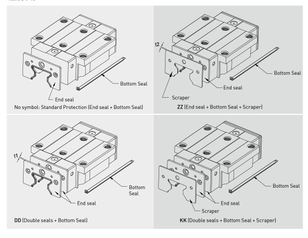
To prevent life reduction caused by iron chips or dust entering the block.
