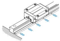
5 Tighten the mounting bolts with a torque wrench to the specified torque.
