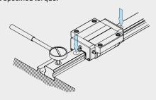
6 Install the remaining linear guideway in the same way.
