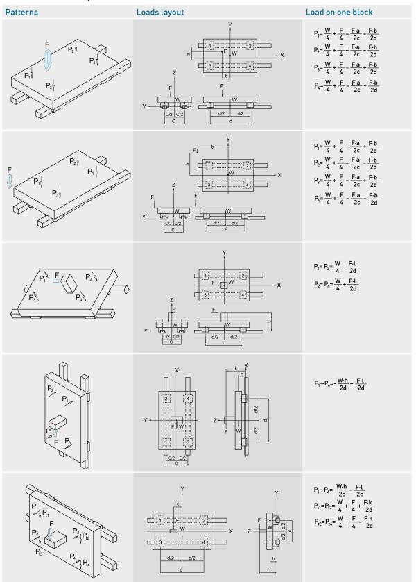
W: Applied weight l: Distance from external force to driver c: Rail spacing
