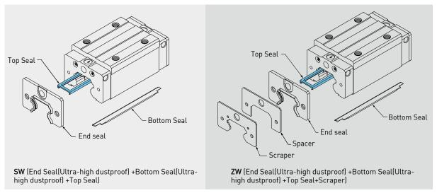
$Note: 1. \ The \ available \ size for \ high \ dust \ proof \ accessories \ are \ HG15C, \ HG20(C/H), \ HG30(C/H), \ HG35(C/H), \ HG45(C/H).$
