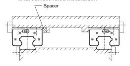
HGW type block with mounting holes in different directions.
