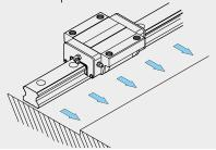
3 Check for correct thread engagement when inserting a bolt into the mounting hole while the rail is being placed on the mounting surface of the bed.
