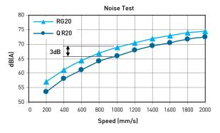
(3) Smooth Movement In standard linear guideways, rolling elements on the load side of the guide block begin rolling and push their way through the raceway. When they contact other rolling elements they create counter-rotational friction. This results in a great variation of rolling resistance. The QR linear guideway, with SynchMotion™ technology prevents this condition.
