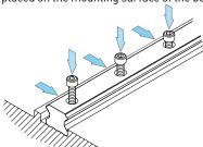
4 Tighten the push screws sequentially to ensure close contact between the rail and the side datum plane.
